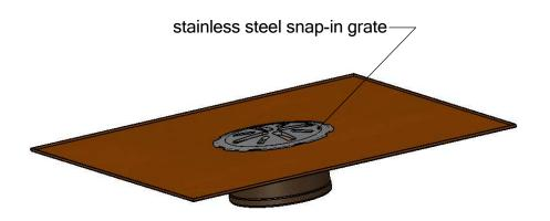
16 oz copper flashing attached to 2", 3" or 4" bronze fitting (2" threaded fitting also available)
